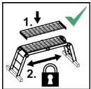
If the ladder is being used as a platform, only decks recommended by the ladder manufacturer may be used. The deck must be secured before use (only if necessary due to the design of the ladder).
