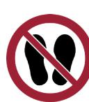
The part of the ladder with this sign is not allowed to stand on.
