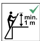
Ladders used for access to a higher level shall be extended at least 1 m above the landing point and secured, if necessary.
