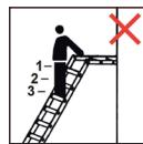
Do not stand on the top three treads/rungs of a leaning ladder.
